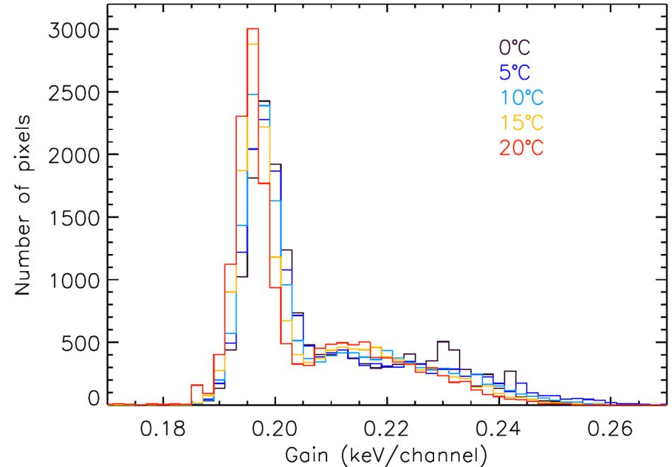
Spectra acquired with Am, Cd, and Co at different temperatures: Fit to each of 16384 pixels to give gain and offset at each temperature
