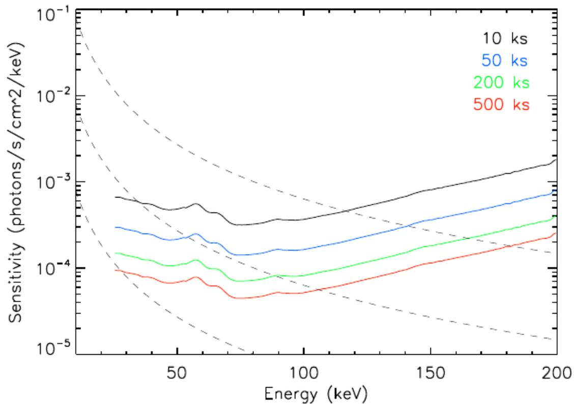
With the new background subtraction technique, the spectroscopic sensitivity is now limited only by statistics for typical observations with exposures up to ~ 500 ks
