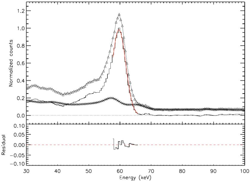
Module wise alpha tagged Am-241 spectra for each month fitted to get peak energy
