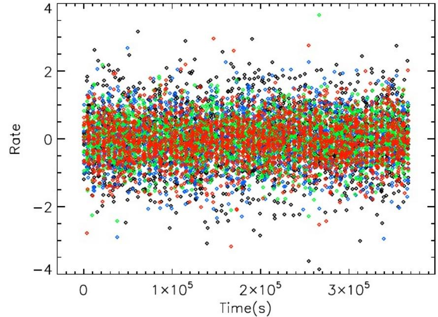
Mask-weighted light curves and spectra consistent with zero for blank sky observations of 200 ks exposures
